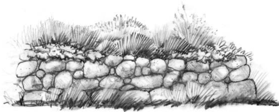
Figure 2.5b - Retaining Wall Finishes - Stacked Wall
